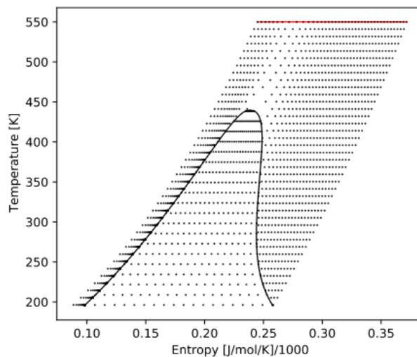
Figure 14: 1233zd R gas T-s diagram
