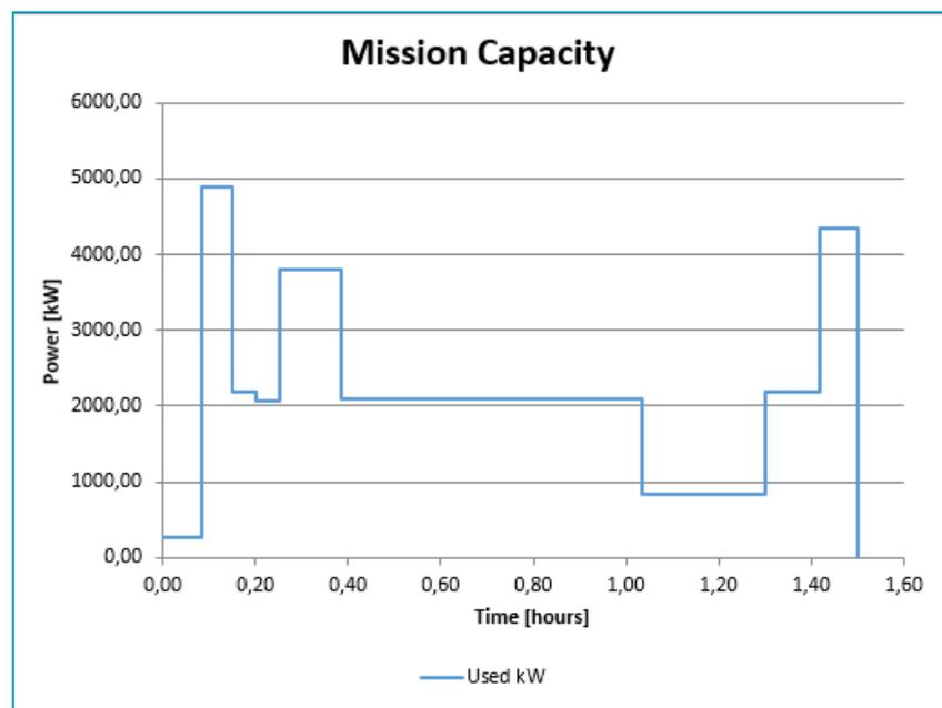
Figure 6: Capacity flight mission graph
